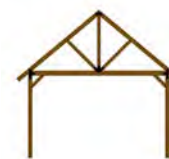
King-Post with Struts Truss
